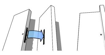
LAMELLO Unlike traditional cam fixings, the fixings we use are designed not to be seen when the unit is assembled. To fit them, simply align the pair of fixings, and use an allen key in the adjacent hole to join twist the lever from one into the other.
